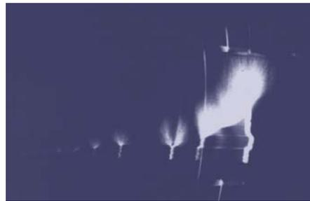
Triggering time of a simple rod lightning conductor
